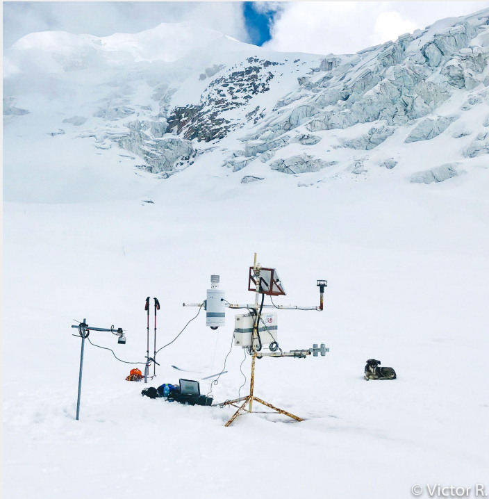
Figure 3 : Automatic weather station on Zongo glacier (SAMA) located around 5050m high, measurement of albedo, temperature, humidity, wind, shortwave and longwave fluxes (in and out).
